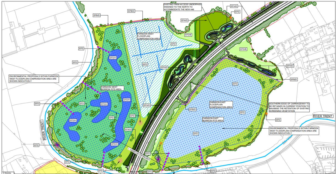
Figure 1 Indicative locations of fish escape passages (dashed pink line) from Farndon flood compensation areas to the River Trent, as detailed in the Environmental Masterplan (AS-026).
